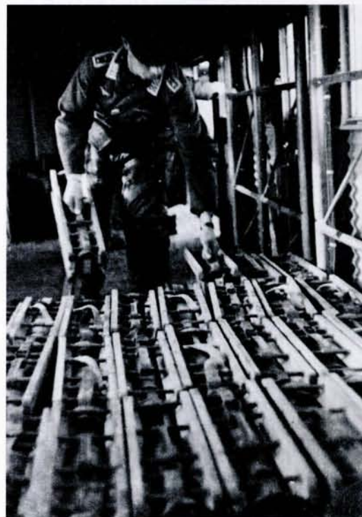
LEFT AND FAR LEFT: The useful load of a Ju 52/3m was up to 2,000 kgs. Here, Panzerfauste and small arms ammunition are being carried aboard a Ju 52/3m where (LEFT) a Luftwaffe Oberfeldwebel stacks the Panzerfaust containers inside the fuselage. Note the machine gun mounted to fire through the fuselage window in the photograph (FAR LEFT).
