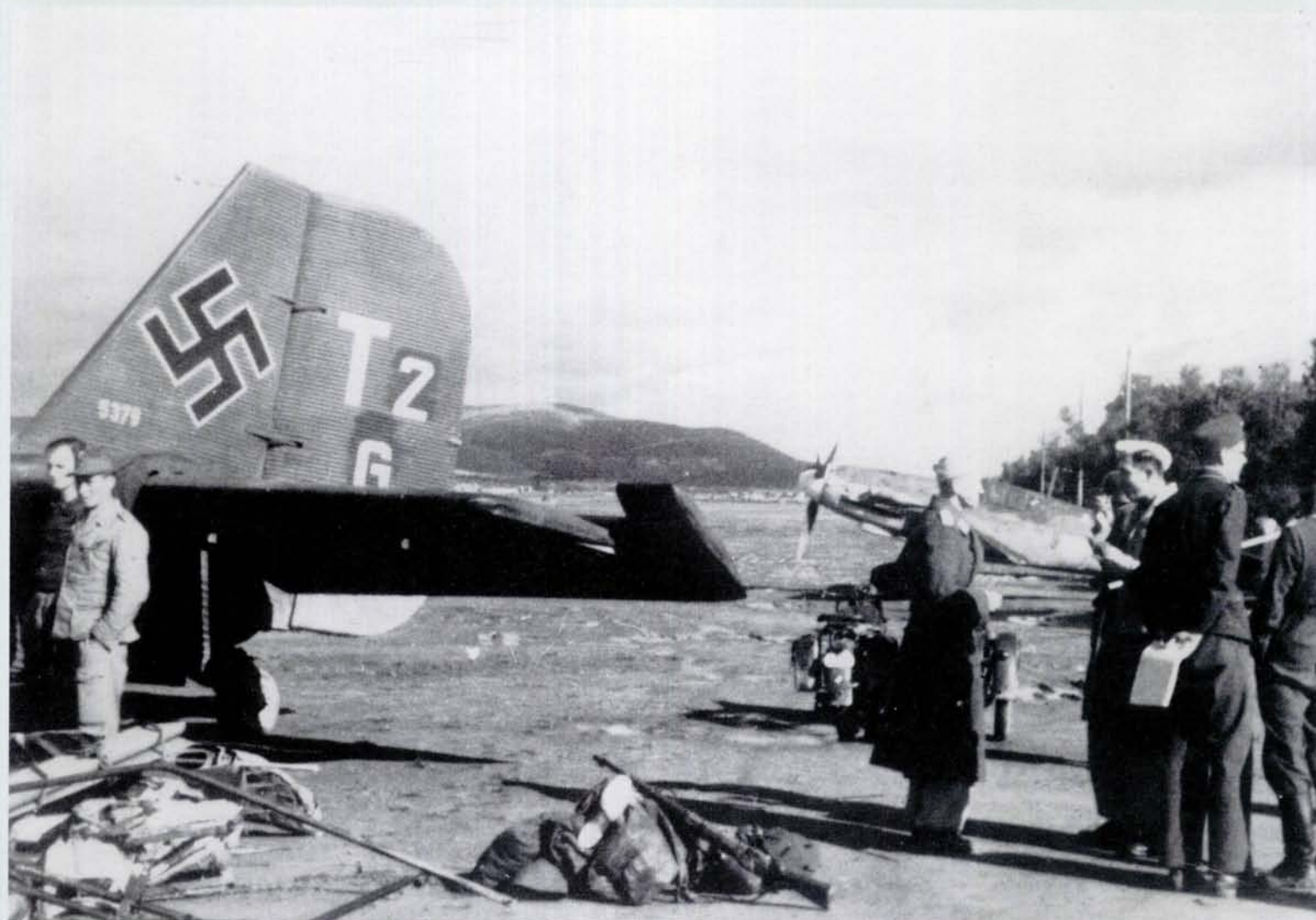
ABOVE: Tactical markings on a Ju 52/3m W.Nr. 5379 at Rhodes in March 1943. Reference to the table on pages 116/117 will show that the large letter 'T' was used at that time by KGzbV 800. The 2 is the Staffel number and the small 'G' the individual aircraft letter.
