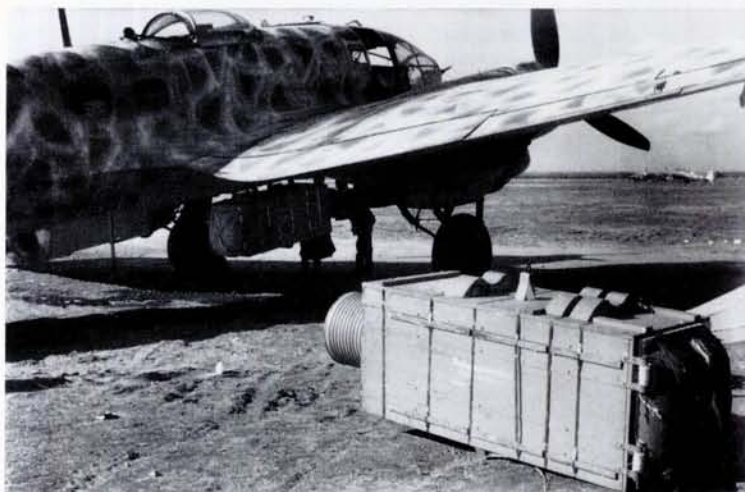
An He 111, probably of TGr 30, with a supply container already mounted beneath the centre section and another in the foreground. Note the winter camouflage, which has been achieved by spraying white or RLM 76 over the original 70/71 finish in such a manner that patches of the original greens appear as mottles. In the spring of 1944, TGr 30 flew 1,285 missions during the operation to supply First Panzer Army encircled near Kamenets-Podolski.
