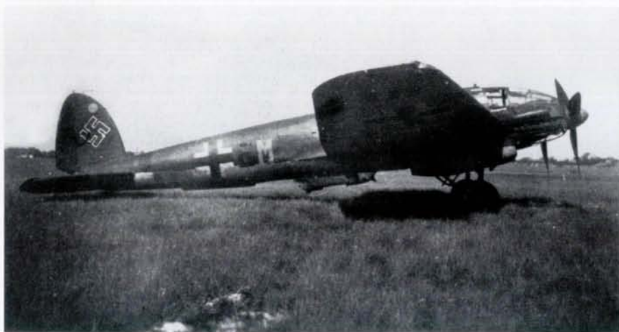
ABOVE AND ABOVE RIGHT: This He 111 H-6 of 4./TG 30 landed at Mönchengladbach on 6 May 1945, when the crew and passengers surrendered to US forces. The machine was finished in a conventional 70/71/65 camouflage but with the Staffel letter 'M' in the operational markings S3+EM finished in blue, the Staffel colour, whereas the normal practice was to paint the aircraft letter in the Staffel colour.
